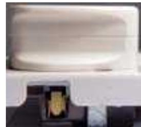
contact is actually squeezing the shaped end of the plastic pin, instead of exerting a firm grip on the straight sides. This often results in “pop out”, the socket cover being pushed slightly out
