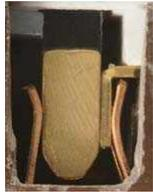
in use in Britain, all work properly with plugs, but often not with socket covers. We cut away a typical 13 Amp socket to show how the pin of the real plug fits into the socket. A close-up of the same plug and socket, shows how the pin fills the contact. Apart from ensuring the electrical connection the socket's contacts serve to hold the plug in place in the socket. This close-up of the socket with a cover inserted shows how the pin is too short to be gripped by the contact. The spring
